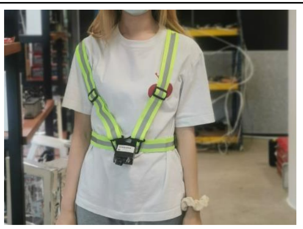
Figure 2.2.2 Actual picture of vest with Beetle and IR Sensors
